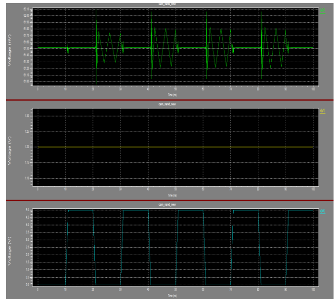
Figure 12:- Output wave form for the GDI based NAND gate design
