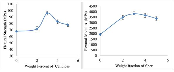
Flexural strength and flexural modulus 2weight percent of jute fiber based composite increased with increase in nanocellulose. The trend variation of flexural strength and flexural modulus is same. Highest flexural strength of 96MPa and flexural modulus of 3807MPa is observed at 3 weight percent of nanocellulose, which is due to good interference and adherence.
