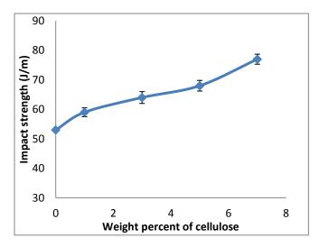
Impact strength of jute fiber based composite increased with increase in weight percent of nanocellulose that is from 2 to 5 weight percent. At 5 weight percent of nanocellulose 77J/m is recorded.
