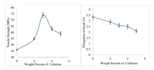
Cellulose of 2, 3, 4, 5 weight percents is incorporated in 2weight percent jute fiber reinforced polyester composite. The tensile strength of composites increased with respect to weight percent of cellulose upto 3 wt% and decreased with further increase in cellulose percent, further. The decline in tensile strength is due to agglomeration of nanocellulose and
