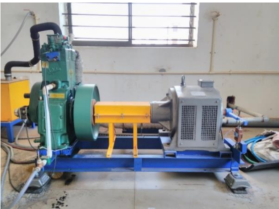
Figure 3.1 singal cylinder 4-stroke diesel engine
