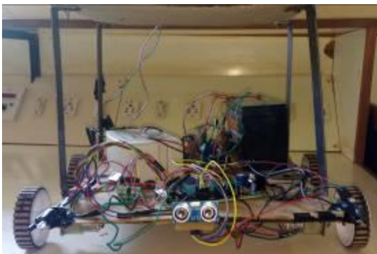
Fig. 7: Practically implemented solar grass cutter
