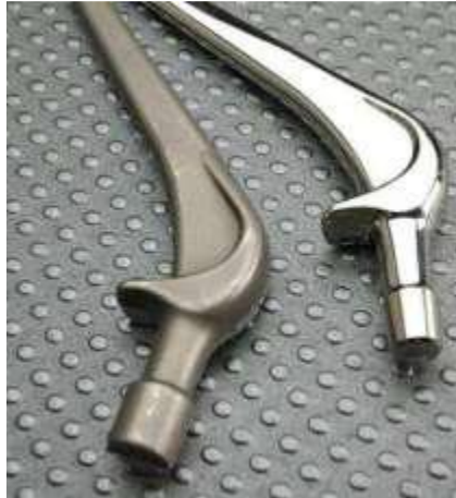
Fig 3.1.2 product before and after finishing
