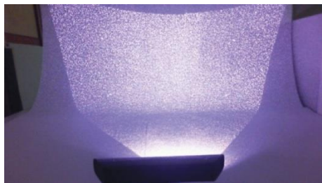
Figure 3: Speckle Pattern from Kinect Sensor
