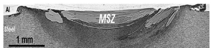
Fig.4. Cross sectional view of an Al-to-steel weld made with  $\omega = 1,400$  rpm,  $v = 20$  mm/min and  $D_p \approx 0.3$  mm displaying MSZ
