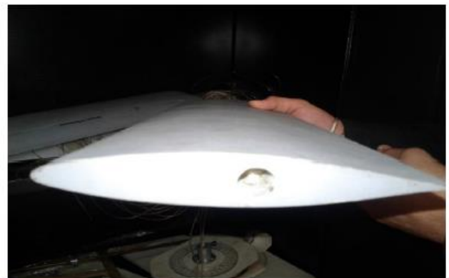
Fig 1.1. wing section with aerofoil NACA 66015
