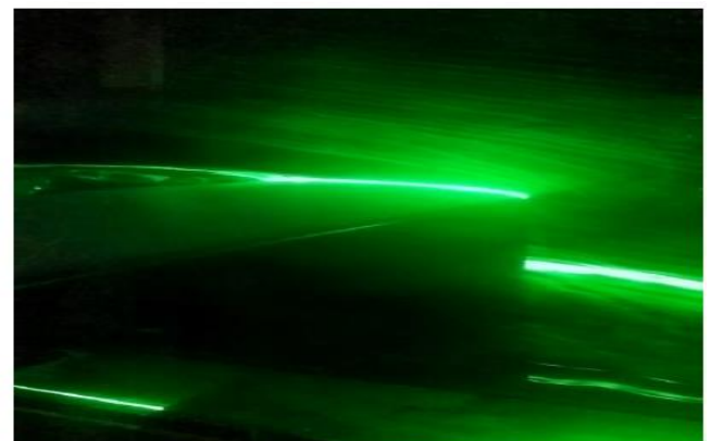
Fig. 4.1 Angle of attack 9 with flap at five degrees
