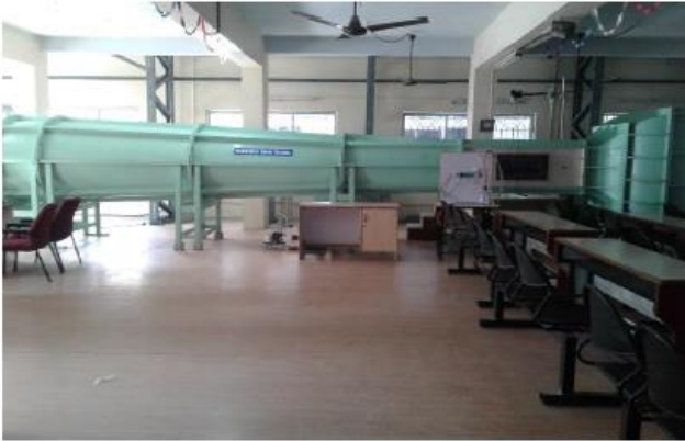
Fig 2.1 subsonic wind tunnel
