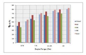
Figure 6: Relationship b/w Mechanical Efficiency and Engine Torque for Different Fuel Blends
