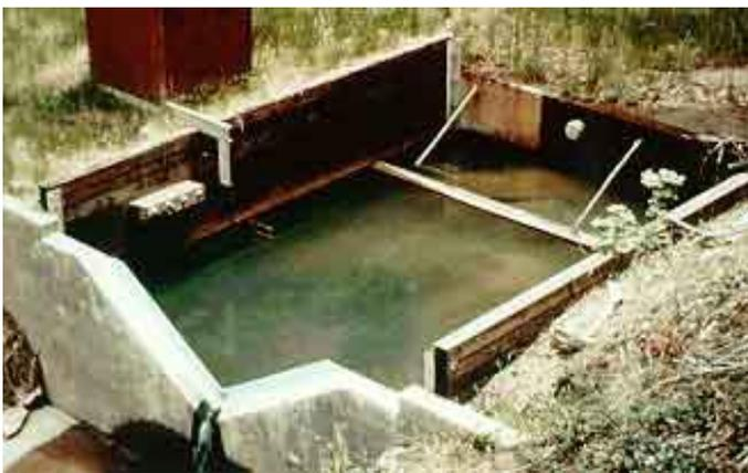
The picture above shows a V-notch weir. The edge the water cascades over is called the crest and the overflowing water sheet is called the nappy. Today weirs are still used to determine flows from open water sources such as streams. A typical 90° V-notch will be beveled at 45° so the edge is less than 0.08” thick and the angle of the notch will be precisely 90°. Water flow over the weir is calculated by the equation:
