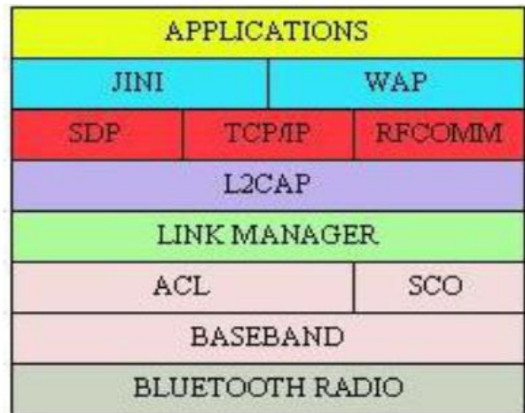
Fig 3. Bluetooth Protocol Stack
