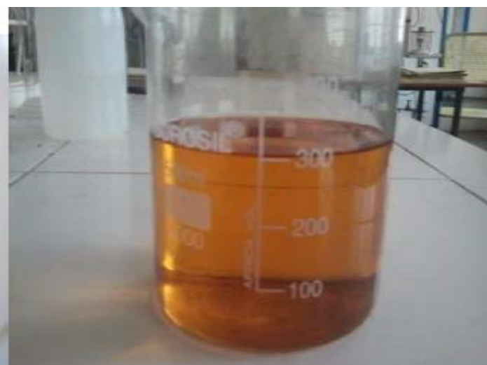
Fig. 5: Product 1 –Below 180 °C (extracted - 20%) Product 2 –Between 210-340 °C (extracted - 34%) Product 3 –Residue (Tar 46%)
