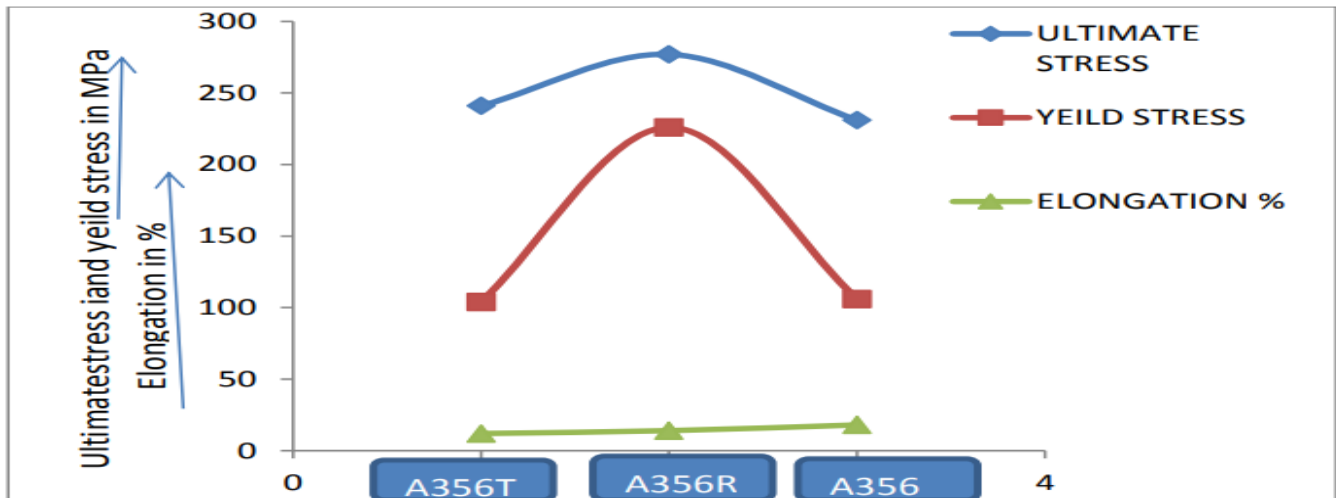
Figure 5: Ultimate Stress, Yield Stress, and Percentage of Elongation Curve of A356 Alloy Under Thixocasting, Rehocasting, and Melting Condition
