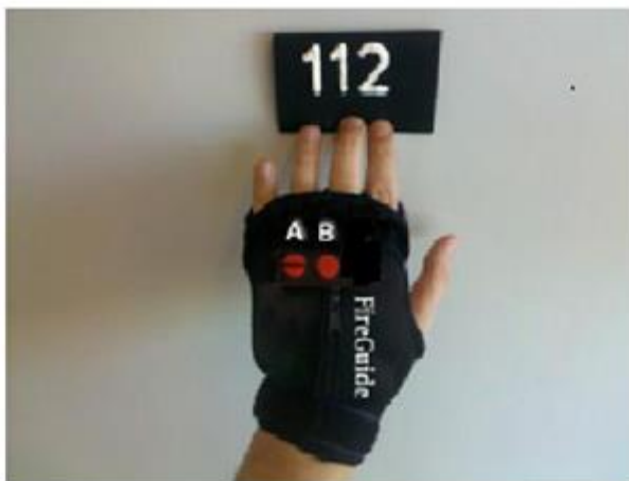
Fig 2: RFID Glove (back view) Scanning an R-Tag
