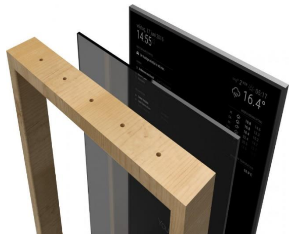
Fig 1:- Architecture of Smart Mirror
