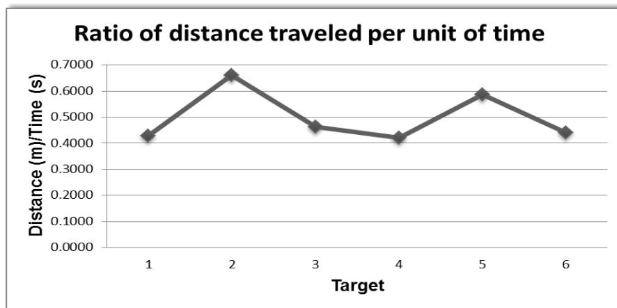
Fig 9:- Average Speed of the Wheelchair using Conventional Wheels
