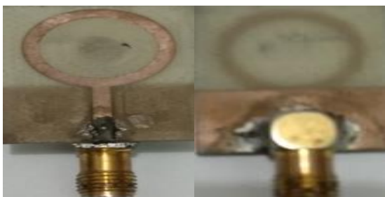
Fig. 10:- Top and bottom view of prototype CRMA
