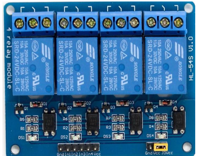
Fig 2:- Four channel relay module
