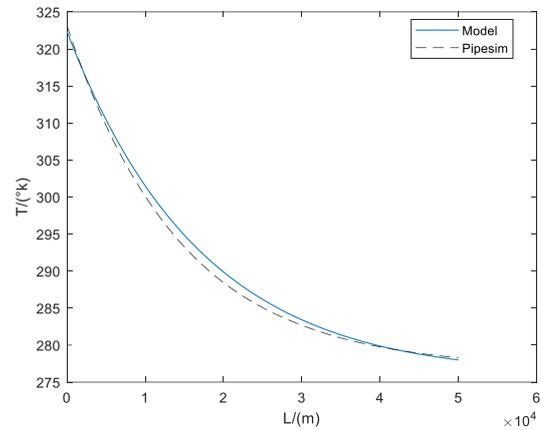
Fig. 4:- Temperature profile comparison between our model and pipesim model.
