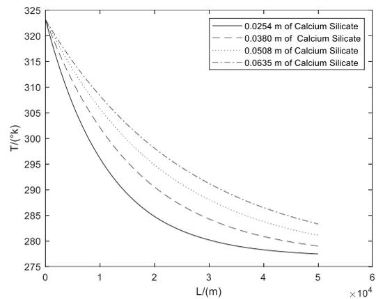
Fig. 9:- Effect of several thickness of calcium silicate on the temperature profile of oil and gas flowing through offshore pipeline of 50 km
