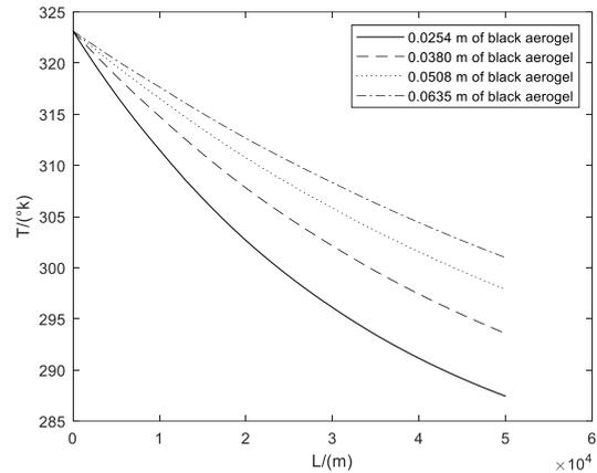
Fig. 8:- Effect of several thickness of black aerogel on the temperature profile of oil and gas flowing through offshore pipeline of 50 km.
