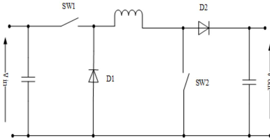
Fig 3:- Non-Inverting Buck Boost Converter
