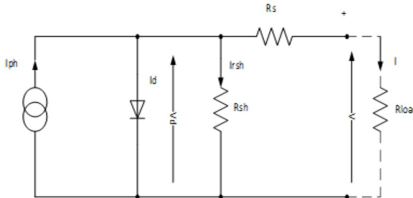
Fig 2:- Single Diode Model
