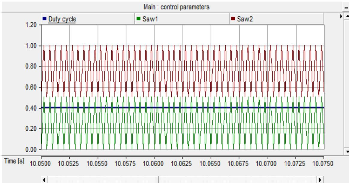
Fig 5:- Duty Cycle, Saw1 and Saw2 Signals for Transistors Firing Pulse Generation
