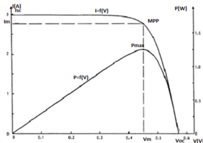
Fig 1:- The Current - Voltage and Power-Voltage Characteristics of a Photovoltaic Cell
