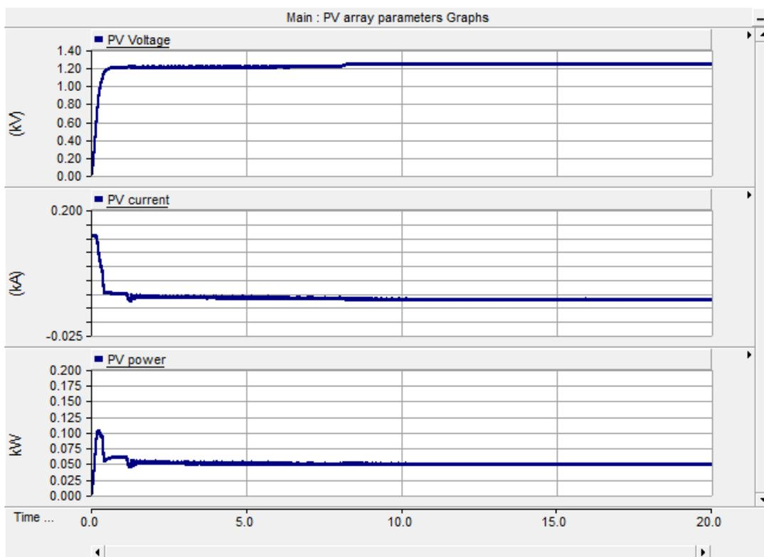
Fig 8:- The Voltage, the Current, and the Power Curves of Photovoltaic Panels
