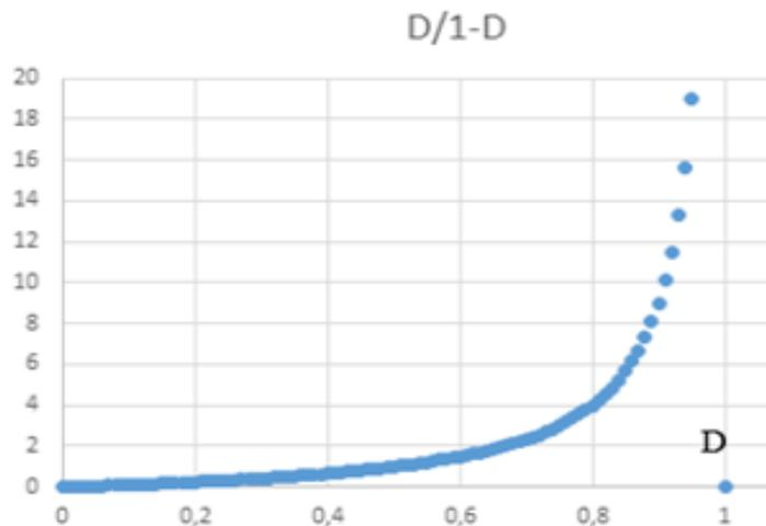
Fig 4:- The Evolution of the Ratio  $V_{out} / V_{in}$  as a Function of the Duty Cycle
