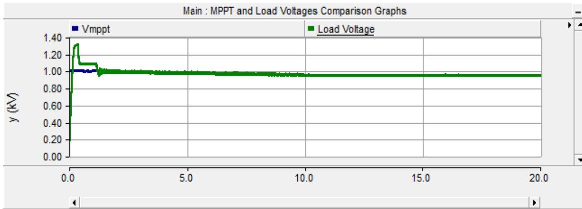
Fig 9:- Comparison Curve of Vmppt Voltages and the Converter Output Voltage
