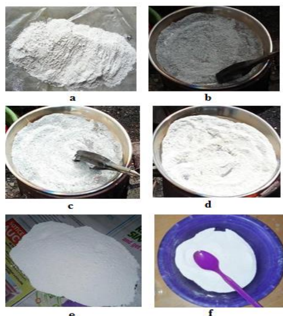
Fig 2:- Eggshell Powder Before Calcined (a) and Eggshell Powder After Calcined at Various Temperature (b) 600 °C, (c) 700 °C, (d) 800 °C, (e) 900 °C, and (f) 1000 °C.
