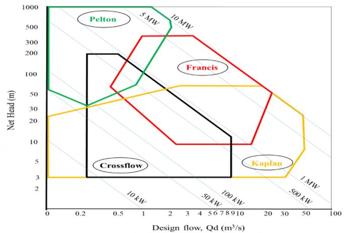
Fig. 4:- Turbine selection chart according to the net head and flow rate
