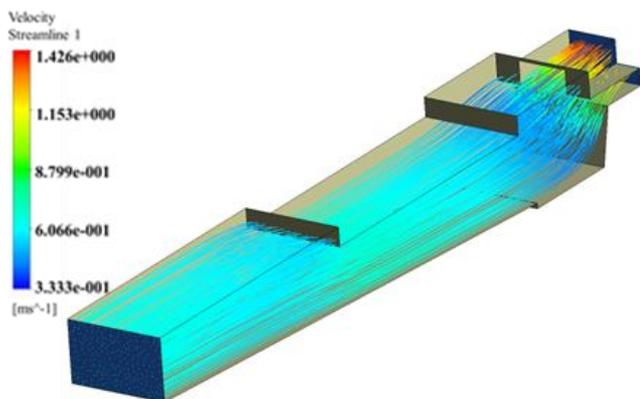
Fig. 31:- Water flow velocity distribution in settling basin (CFD simulation).
