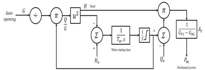
Fig. 9:- Turbine model schematic diagram
