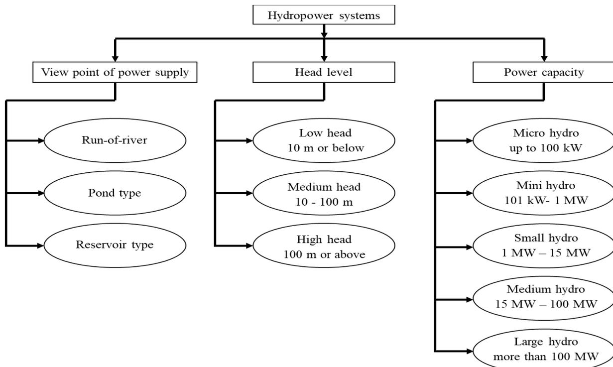
Fig. 1:- Complete classifications of hydropower systems.
