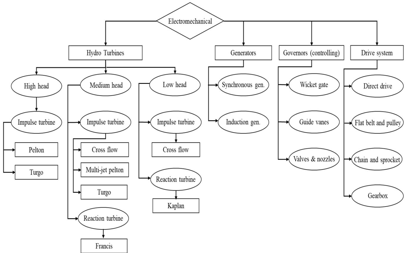
Fig. 3:- Electromechanical equipment of HPP
