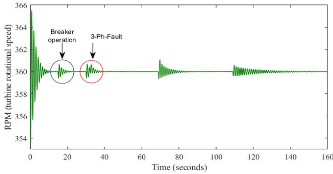
Fig. 22:- RPM response during the HPP operation
