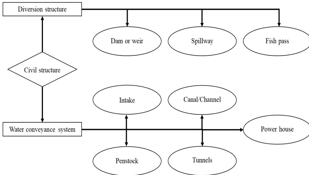
Fig. 2:- Hydraulic structures in HPP.
