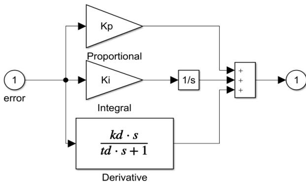
Fig. 6:- PID controller design.
