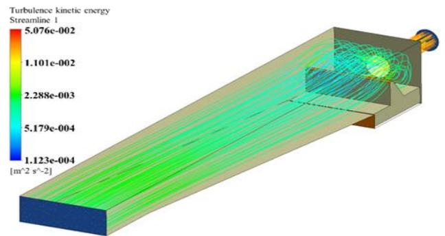
Fig. 26:- Turbulence of kinetic energy in fore-bay (CFD simulation).
