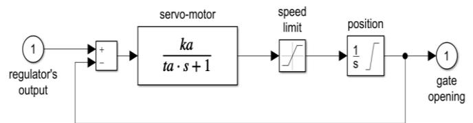
Fig. 7:- Servo gate operation controller design
