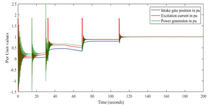
Fig. 21:- Power generation, Excitation current and Intake Gate positions n in Per Unit values
