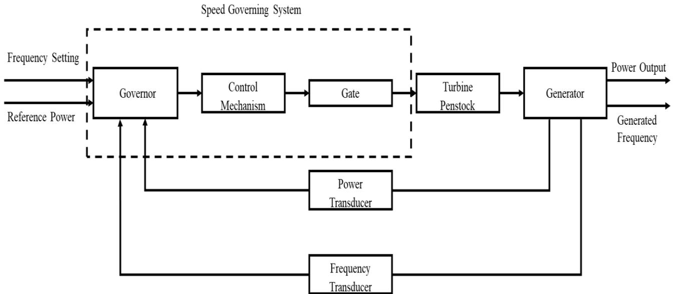
**Fig. 5** Block diagram of a Hydro power plant operation
