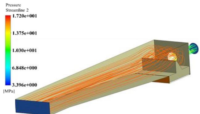
Fig. 28:- Pressure induced in fore-bay (CFD simulation).
