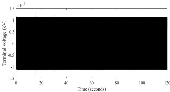
Fig. 23:- Regulated 11 kV voltage at terminal with respect to the power generation.
