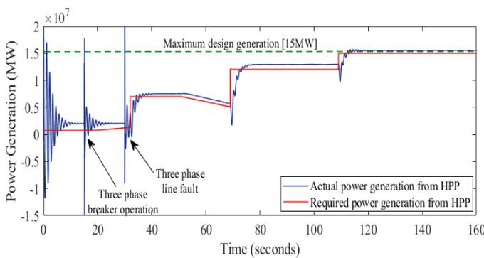
Fig. 18:- HPP actual generation Vs required generation comparison
