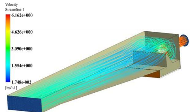
Fig. 27:- Water flow velocity distribution in fore-bay (CFD simulation).
