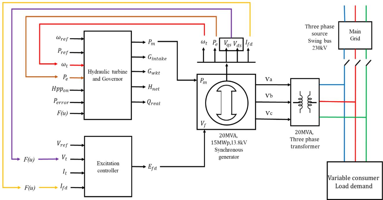
Fig. 11:- Grid connected hydropower station schematic diagram
