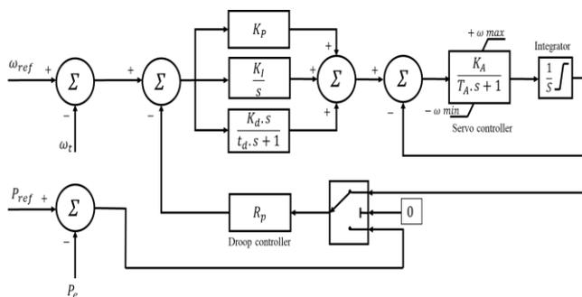
Fig. 8:- Speed regulation controlling schematic diagram.
