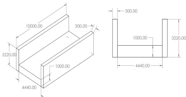
Fig. 13:- Headrace open channel design
