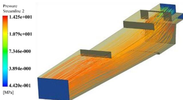
Fig. 30:- Pressure induced in settling basin (CFD simulation).
