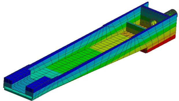
Fig. 25:- Hydropower structure deformation analysis in ANSYS.
