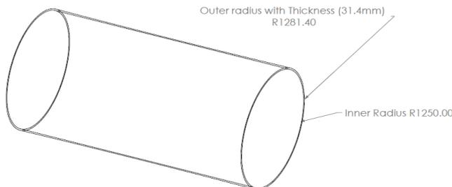
Fig. 16:- Penstock pipe dimensions
