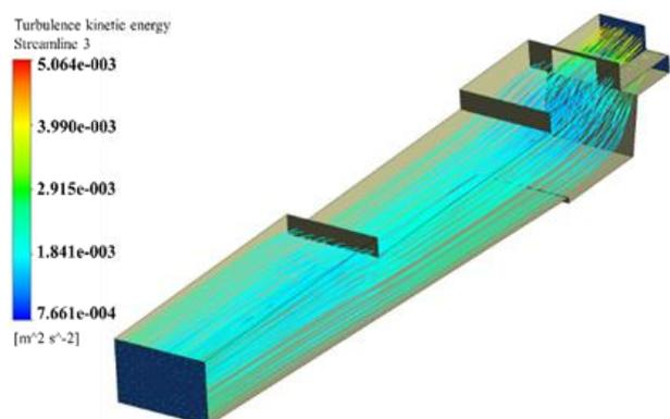
Fig. 32:- Turbulence of kinetic energy in settling basin (CFD simulation).
