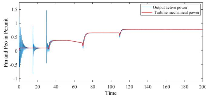
Fig. 19:- Power generation tracking mechanical power variation.
