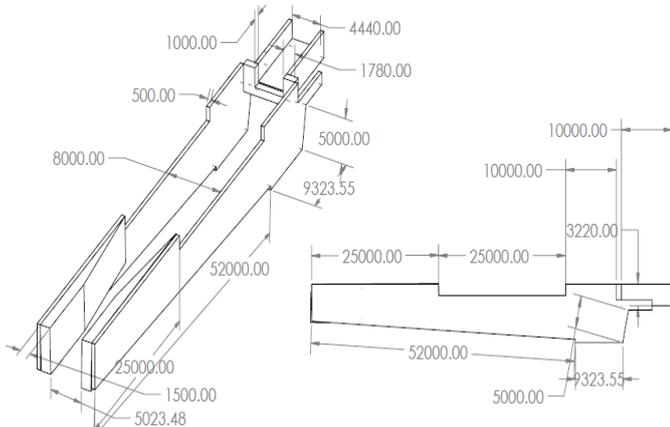
Fig. 12:- Settling basin design
