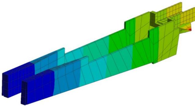
Fig. 29:- Settling Basin structure deformation analysis in ANSYS.
