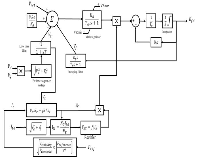
Fig. 10:- Excitation schematic diagram.
