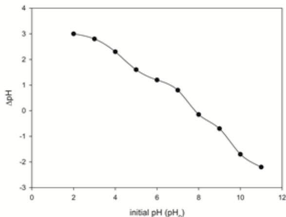
Fig 2:-  $pH_{ZPC}$  of Activated carbon
