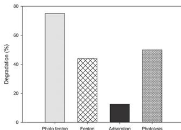
Fig 3:- Preliminary experiments of photo-Fenton, Fenton, adsorption and photolysis under identical experimental conditions at MO initial concentration= 5mg/L, Fe-Ac dose = 1.0g/100mL, pH = 3 and H<sub>2</sub>O<sub>2</sub> = 1.0mL for 30 minutes
