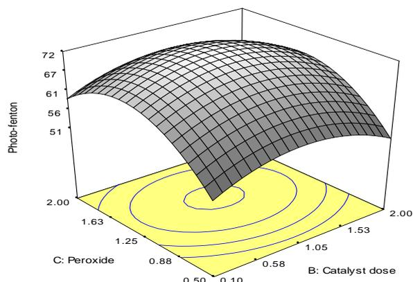
Fig 4:- Interaction plot of reaction parameters
