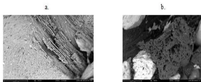
Fig 1:- SEM image of Activated Carbon
