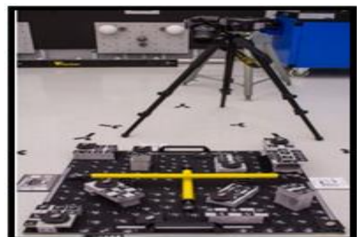
Figure 5 3D test object consisted of about 170 coded targets with a largest dimension of 900 mm.
