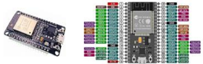
Fig 1:- Espressif ESP32 microcontroller and its pin configuration
