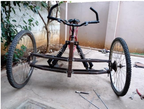
Fig 5:- Final assembled reverse electric trike
