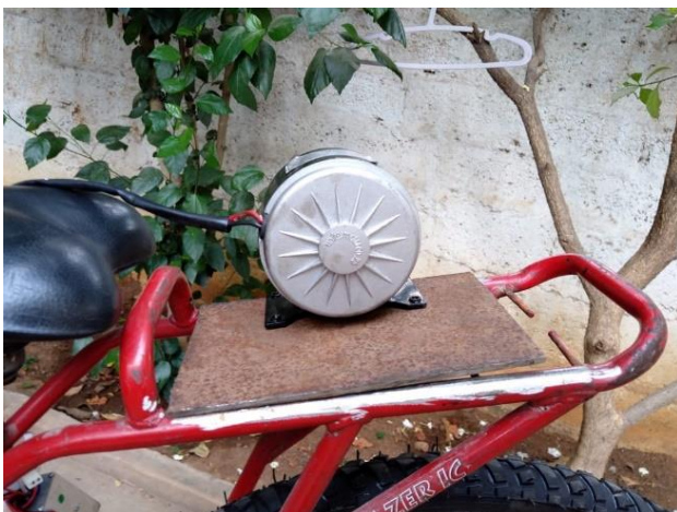
Fig 6:- BLDC Motor mounting on the cycle
