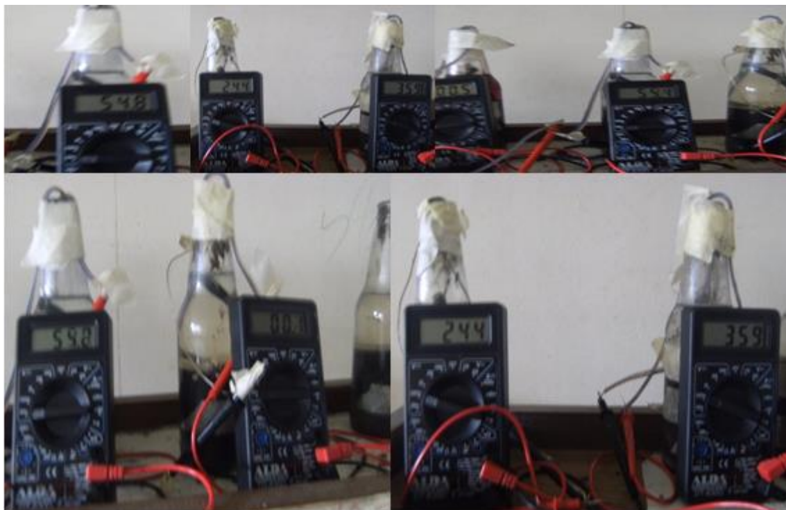
Fig. 2:- Functioning Sediment Microbial Fuel Cells in a Bioelectrochemical remediation
