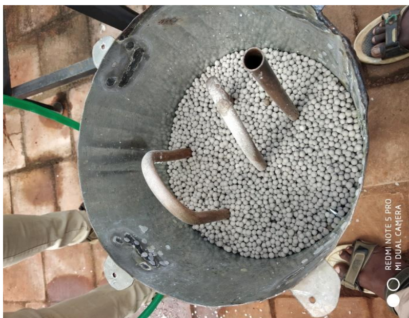
Fig. 2:- Energy storage setup filled with energy storage material(Zeolite)
