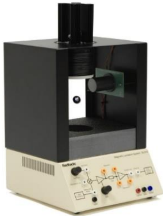
Fig 1:- Magnetic levitation experimental system
