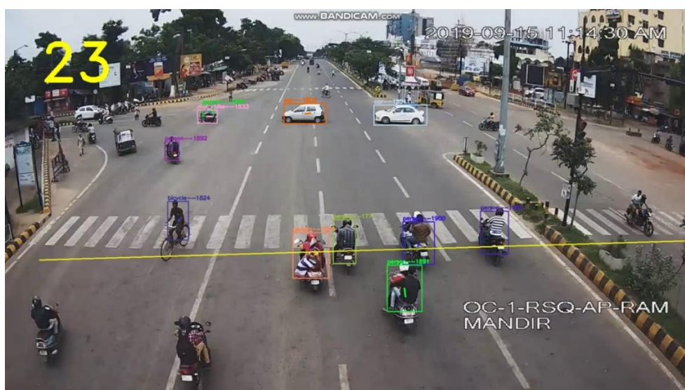
Fig 5:- Parsing class names using the proposed algorithm, courtesy: Bhubaneswar Smart City Limited
