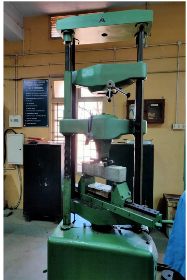
Fig 5:- Experimental setup for flexural strength test.
