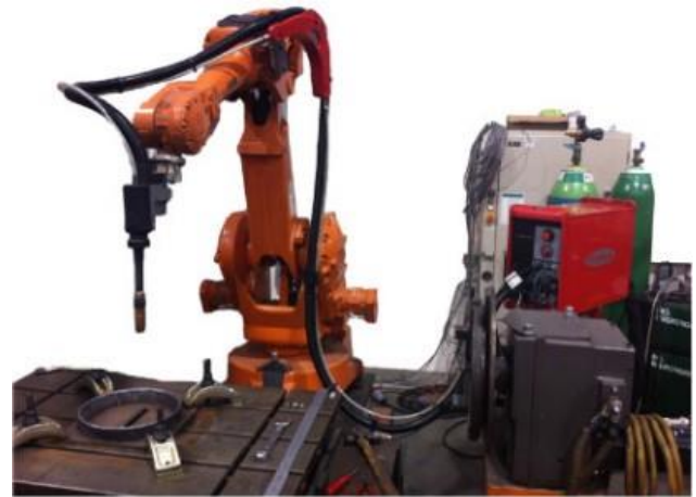
Fig. 4:- A standard automatic-WAAM setup [4]
