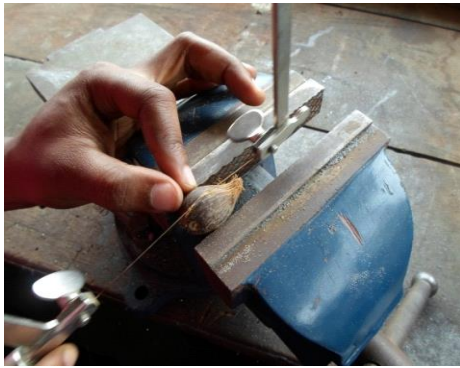
Plate 5: Sawing with the jewellers' saw
