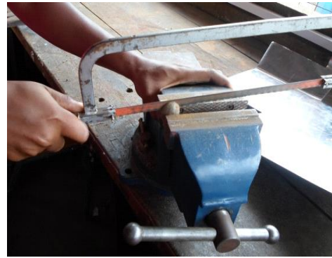
Plate 6: Sawing with the hack saw
