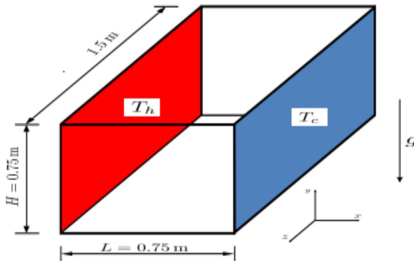
Fig 1:- Geometry of the 3-D numerical model
