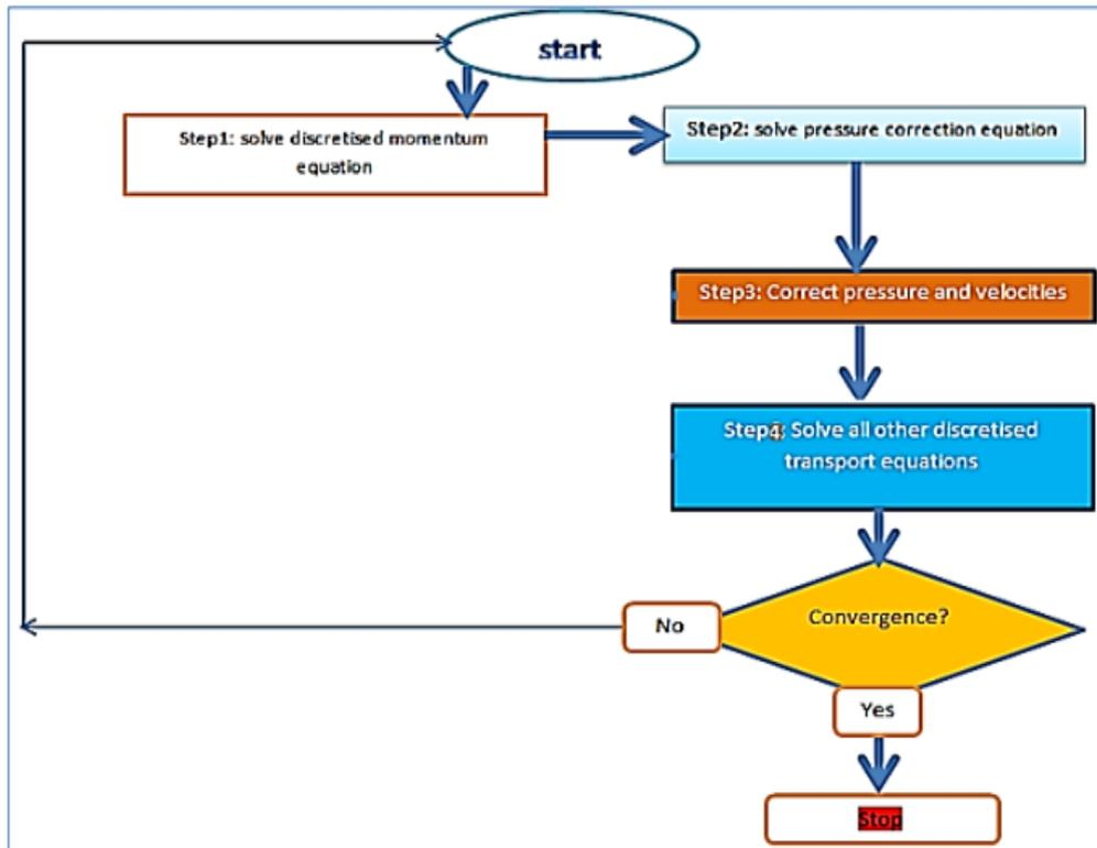
Fig 3:- SIMPLEC Algorithm flow chart
