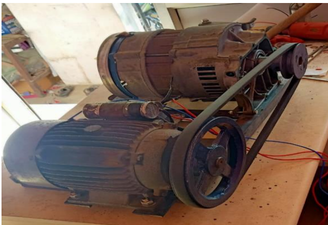
Fig -2: Pulley System
