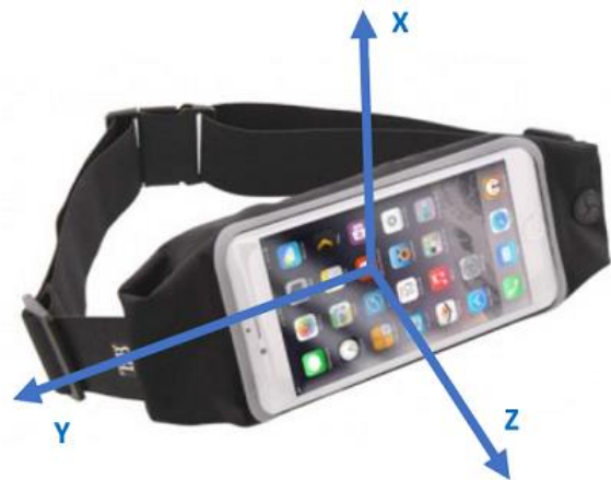
Fig. 1. Axis orientation of the accelerometer embedded in smartphone
