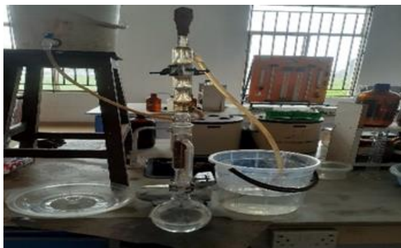
Fig. 1: Soxhlet Extraction setup
