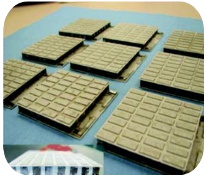
Fig. 4 Skutterudite Thermoelectric Peltier.
