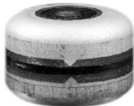
Fig2. General Purpose Heating Source Pallet (Pu 238 ).
