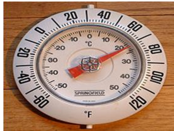
Fig1: thermometer with Fahrenheit (noted on outer dial) & Celsius degree (noted on inner wheel)
