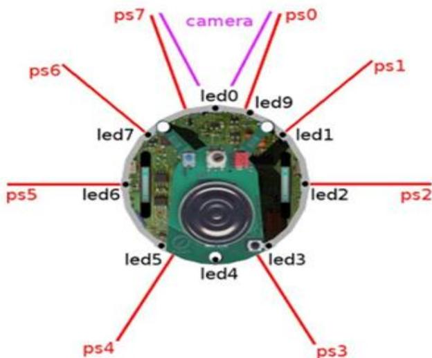
Fig. 5. Sensors, LEDs and camera
