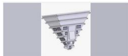
A hopper is a large, pyramidal or cone shaped container used in industrial processes to hold particulate matter or flow-able material of any sort, like dust, gravel, nuts, seeds etc. and can then dispense these from the bottom when needed.
