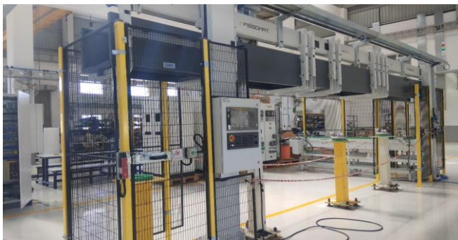
Figure 9: I-Gantry Automation Cell
