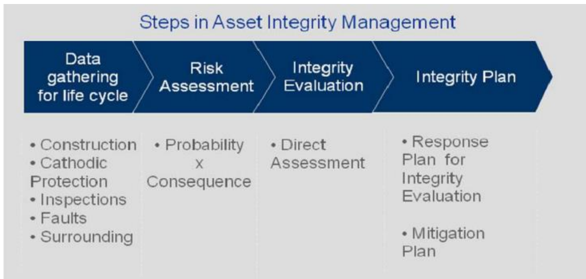
Figure 3 Route for managing asset integrity [8]
