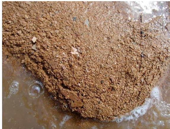
Figure 17 Shredded scale debris after the third MCT cleaning cycle in the 14-inch brine line [28]
