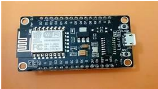
Fig 2: NodeMCU with Wi-Fi Module ESP8266-01.
