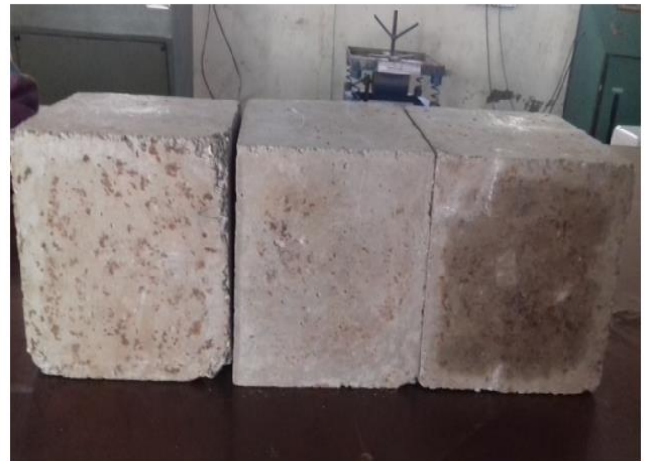
Fig. No 2. Crack Healed blocks.
