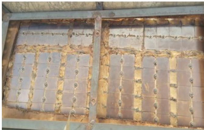
Fig. 5: TEG Peltier distance design two where there's no space in between for the series-connected modules
