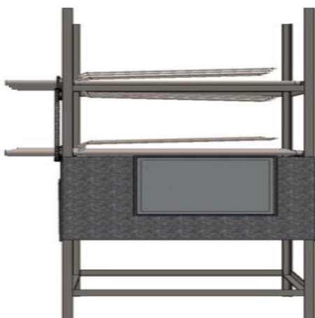
Fig. 2: TEGs Peltier module placed in the wall casing of the grill machine for harvesting of the waste-heat energy
