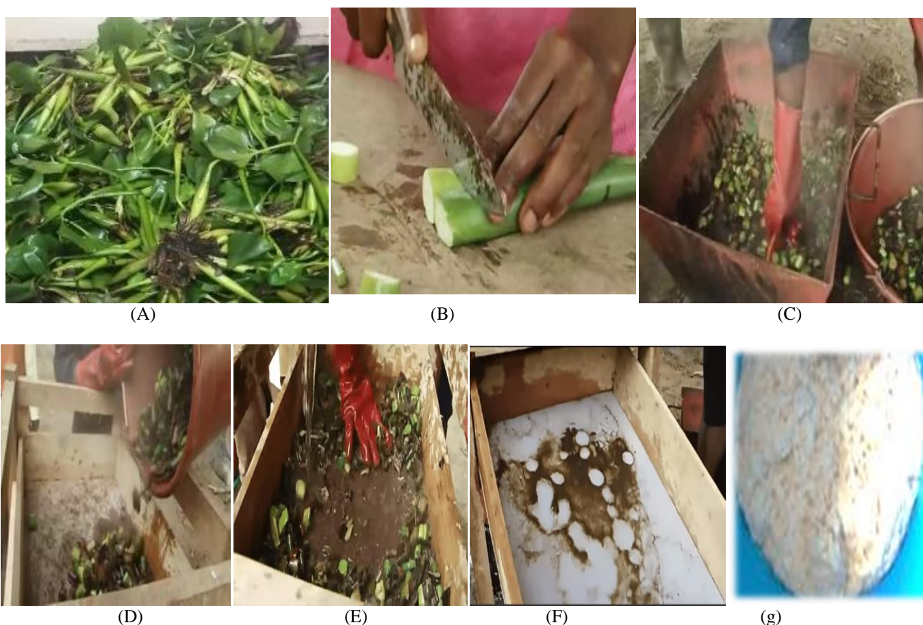
Fig. 2: some pictures of the WH fiber extraction process: (a) WH plant, (b) WH stems harvested, (c) WH boiling, (d) Pouring of WH, (e) Stretching and grinding of WH, (f) WH Brown cellulose extracted, (g) Whitening of the cellulose.
