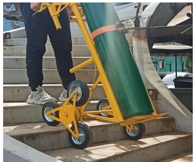
Fig. 7. The prototype climbing the spiral stairs with a 150 mm rise
