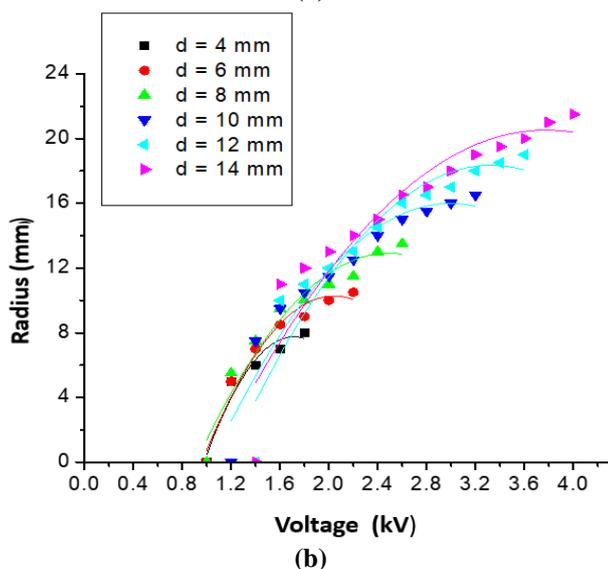
Fig 3:- (a) Used lubricating oil (b) new lubricating oil. The deformation's radius of lubricant oil in EHD phenomenon as function of applied voltage
