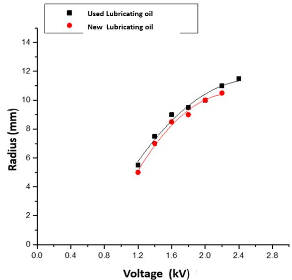
Fig 4:- Radius of circle deformation of used and new lubricant oil as function of applied voltage
