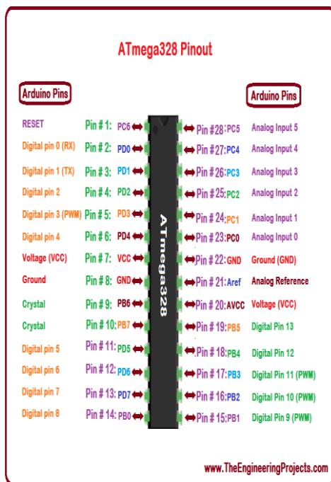
Fig. 4: The Pin-out of ATmega328P Microcontroller
